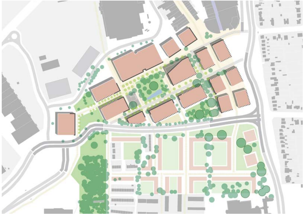
The development framework with active frontages illustrated. Solid lines indicate active frontage and dashed lines indicate passive frontage
