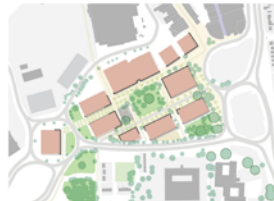
Active frontages illustrated, ensuring the green space and key walking routes are fronted by buildings
